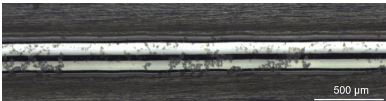
Figure 9: Laser cladded FeCrAl single track on 316L flat substrate.
